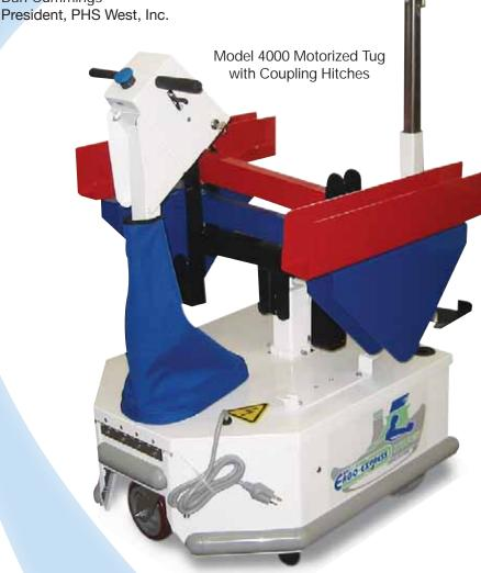
The perfect fit to meet your needs. Our universal coupling hitch allows you to link or "train" multiple carts with no additional hardware required. We can custom design attachments that meet your departmental requirements.
